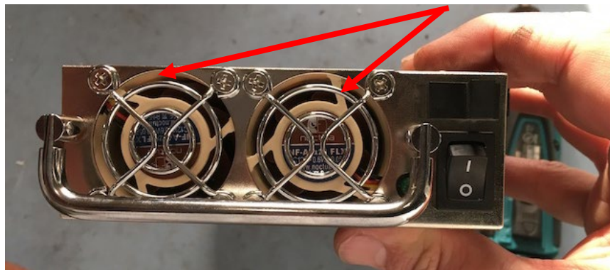
Figure 3: DOMHub ATX power supply module after replacement of both fans.
