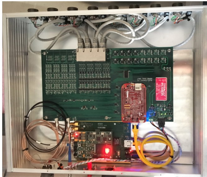
Figure 4: New scintillator central station DAQ electronics (digital readout variant).
