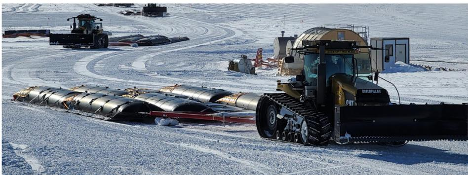
Figure 7: SPOT Tractor hauling 18k bladder set (USAP Photo Library)
