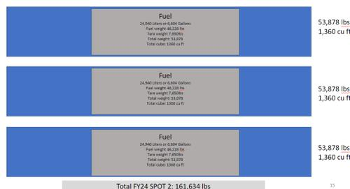
Figure 8: Model of three ISO tank container on SPOT sleds
