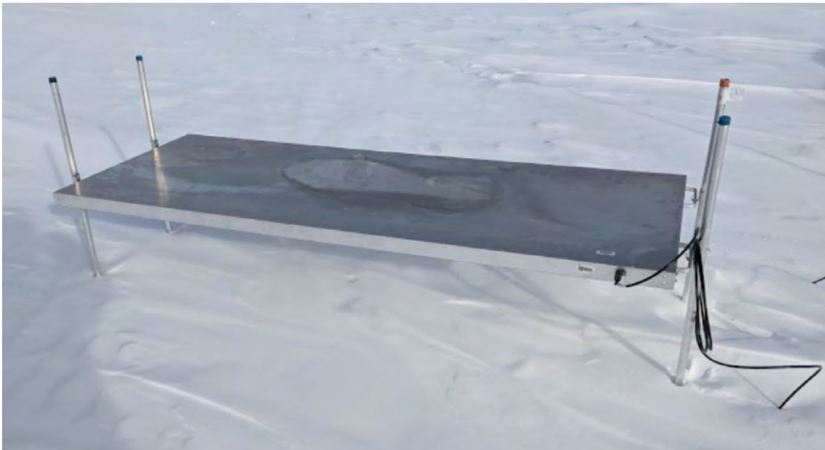
Figure 5: One elevated scintillator panel, close to the snow surface, was raised by the winterovers in early 2022 (photo is prior to raising).
