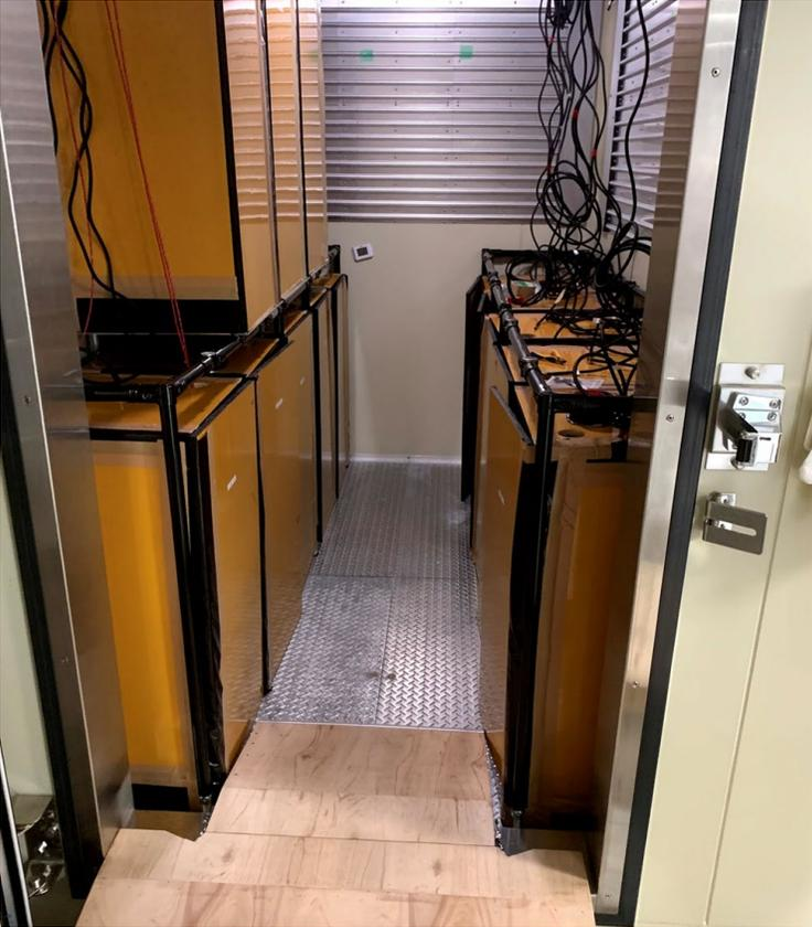
*Freezer partially loaded with D-Eggs in their test structures*
