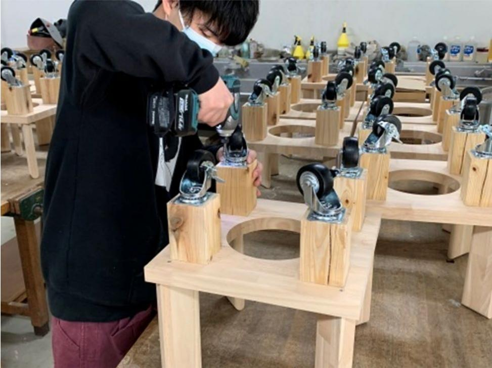
*D-Egg module holders, for the D-Egg FAT, being assembled*
