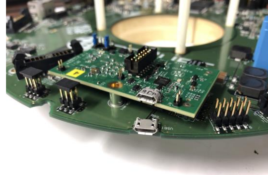
Ice Comms Module on D-Egg Mainboard
