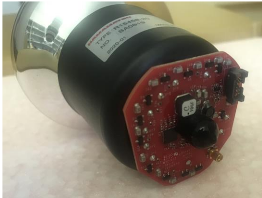
Hamamatsu R15458-20 PMT+ \mu Base Assembly
