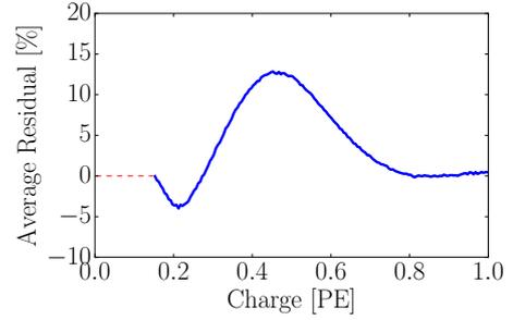
**Figure 4.** The extracted residual in blue, comparing the result of the convolutional fit to the data, averaged over all DOMs. The dashed red line indicates the region where we do not have sufficient data and therefore set the residual to 0% (i.e. no correction will be applied in this region).
