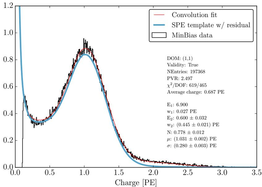
**Figure 5.** An example fit for DOM(1,1) using the MinBias dataset (black histogram) including data from seasons IC86.2011 to IC86.2016. The result of the convolution fit, which includes the 2 PE contribution, is shown as a solid red line and the extracted SPE charge template from the fit is shown in blue. For both the convolution fit and the SPE charge template, the curves include the correction from the average residual shown in Fig. 4.
