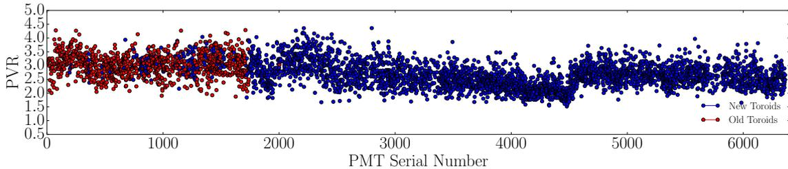
**Figure 7.** The measured peak-to-valley ratio for the standard QE PMTs ordered by PMT serial number. The red data points indicate a PMT instrumented with an old toroid, whereas new toroids are indicated by the blue data points.
