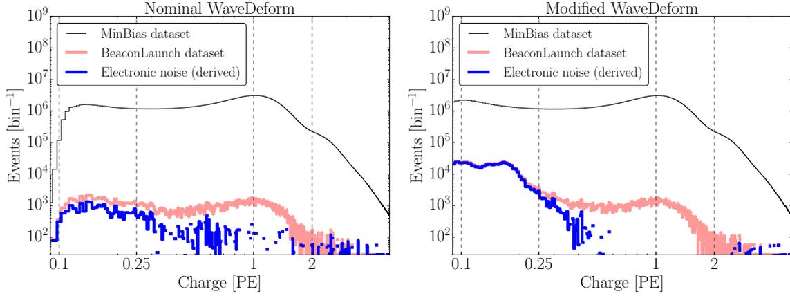
**Figure 3.** The cumulative charge distributions of all DOMs for the MinBias (M) and BeaconLaunch (B) datasets. The blue histogram shows the derived contribution from electronic noise. This was found by subtracting the normalized MinBias dataset from the BeaconLaunch dataset ( $B - M \times (B|_{1PE}/M|_{1PE})$ ). Left: The charge distributions for the standard WaveDeform settings. Right: The charge distributions for the modified WaveDeform settings.
