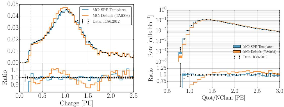
**Figure 10.** A comparison between the SPE charge templates (blue) and the TA0003 (orange) model for describing the SPE charge distribution in Monte Carlo. The simulation is compared to the 2012 IceCube season. The data is shown in black. Left: The total measured charge per DOM, per event at analysis level. Right: The distribution of the total measured charge of an event divided by the number of DOMs that participated in the event.
