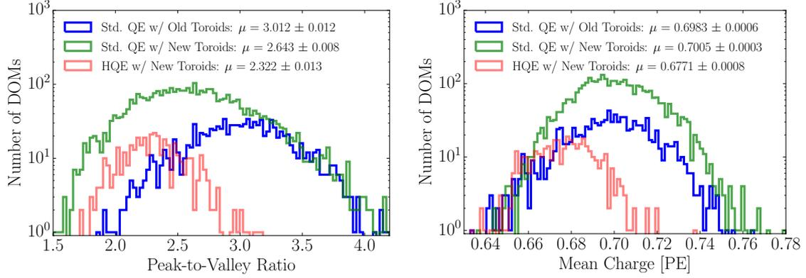
**Figure 6.** Comparison between the R7081-02MOD HQE DOMs and standard R7081-02 DOMs. Left: The peak-to-valley ratio for the two subsets of quantum efficiencies. Right: The average charge of the individual DOM SPE charge templates.
