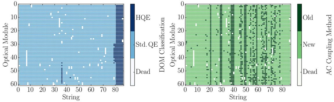
**Figure 1.** Left: A mapping of the HQE (dark blue) and Standard QE DOMs (light blue). Right: The version of AC coupling, old toroids (dark green) and new toroids (light green). DOMs that have been removed from service are shown in white.
