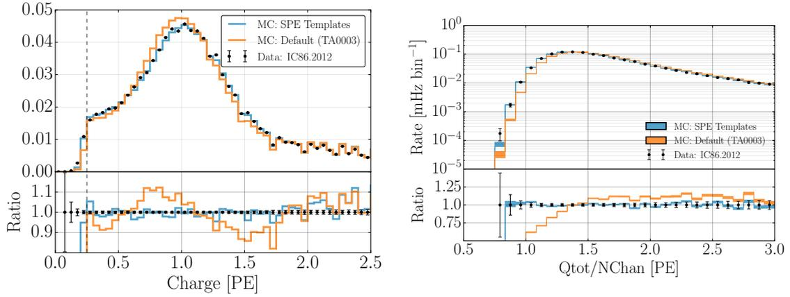
**Figure 9.** A comparison between the SPE charge templates (blue) and the TA0003 (orange) model for describing the SPE charge distribution in Monte Carlo. The simulation is compared to the 2012 IceCube season. Left: The total measured charge per DOM, per event at analysis level. Right: The distribution of the total measured charge of an event divided by the number of DOMs that participated in the event.
