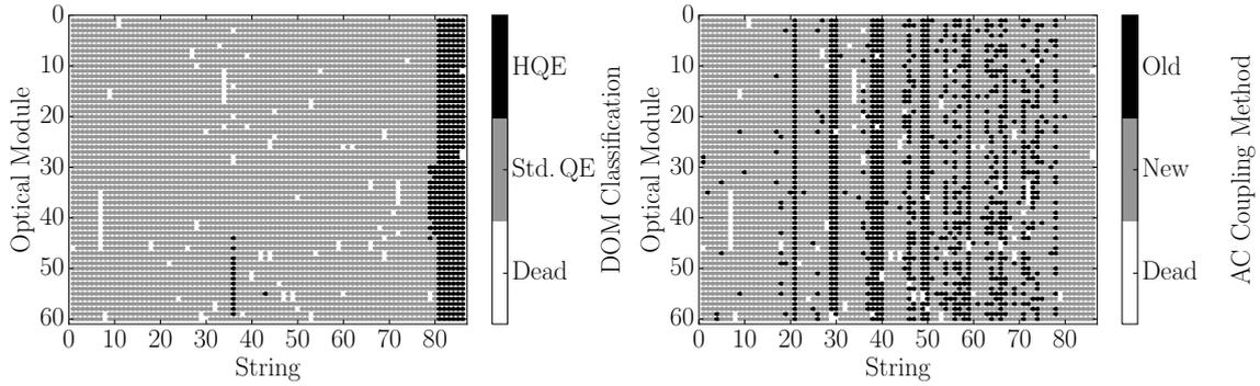
**Figure 1.** Left: A mapping of the HQE (black) and Standard QE DOMs (gray). Right: The version of AC coupling, old toroids (black) and new toroids (gray). DOMs that have been removed from service are shown in white.
