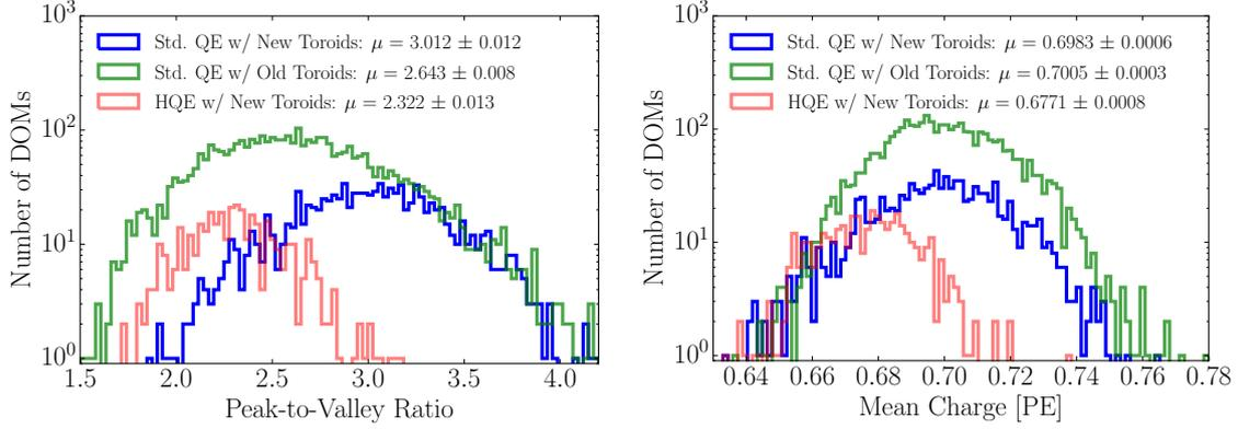
**Figure 6.** Comparison between the R7081-02MOD HQE DOMs and standard R7081-02 DOMs. Left: The peak-to-valley ratio for the two subsets of quantum efficiencies. Right: The mean charge of the individual DOM SPE templates.
