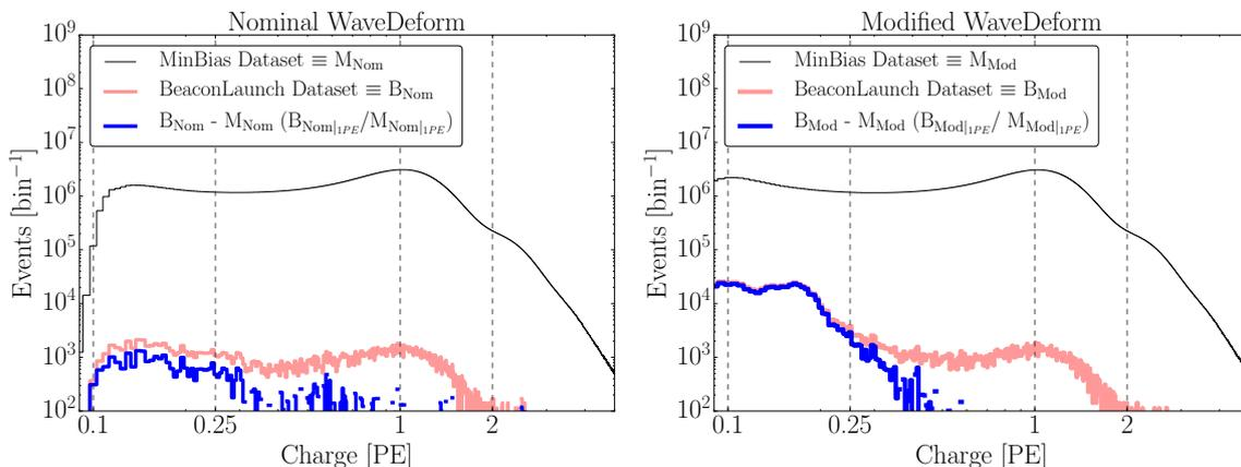
**Figure 3.** The cumulative charge distributions of all DOMs for the MinBias and BeaconLaunch datasets. The blue histogram shows the expected contribution from noise. This was found by subtracting the shape of the MinBias dataset from the BeaconLaunch dataset. Left: The charge distributions for the standard WaveDeform settings. Right: The charge distributions for the modified WaveDeform settings.
