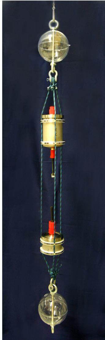
**Figure 2.9:** View of an acoustic SPATS stage. The transmitter module is mounted about 45 cm above the sensor module. The two spacer balls are used to assure a minimum distance of the stage to the IceCube main cable and the wall of the hole. From [100]
