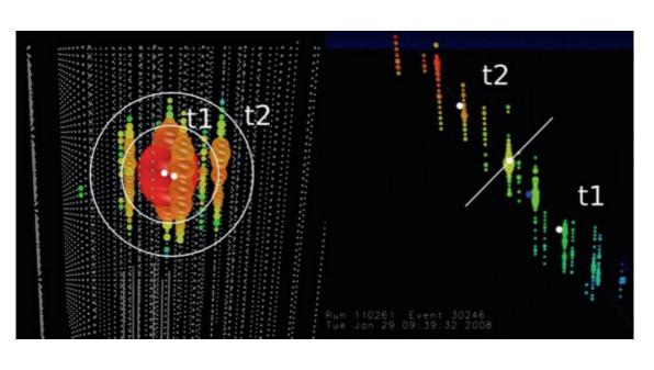
TimeSplitPosition - each event was split into two halves (t<sub>1</sub>,t<sub>2</sub>) based on the charge-weighted mean time, and the cascade reconstruction was run on each half separately. TimeSplitPosition - the difference between reconstructed vertex positions for both halves.
