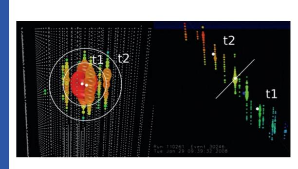
Each event was split into two halves  $(t_1,t_2)$  based on the charge-weighted mean time, and the cascade reconstruction was run on each half separately. Then, the difference TimeSplitPosition between reconstructed vertex positions for both halves was calculated. For the events consistent with a signal cascade hit pattern this number has a smaller value than for track-like events.
