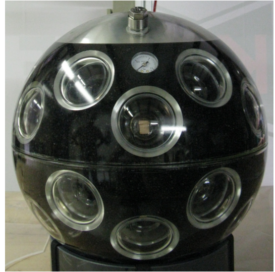
Figure 3: The optical sensor for KM3NeT contains 31 small PMTs (Photo courtesy KM3NeT[8])
