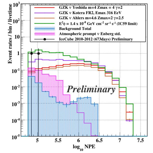
• Observed 2 high NPE events near the NPE threshold
