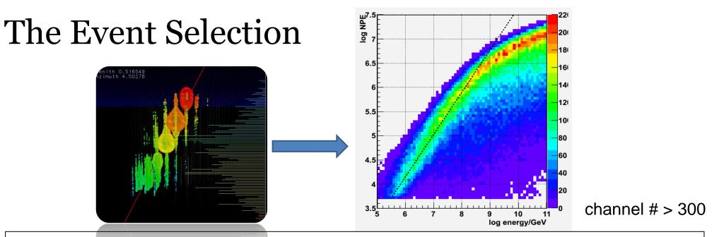
Energy of incoming particle  $\propto$  Energy-losses in detector  $\propto$  number of photo electrons (NPE)
