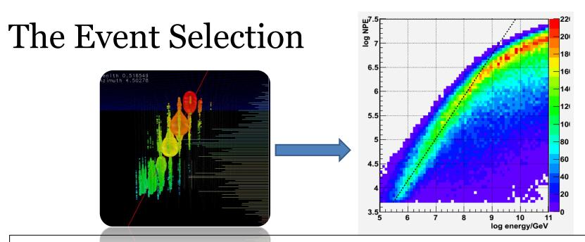
Energy of incoming particle ∝ Energy-losses in detector ∝ number of photo electrons (NPE)
