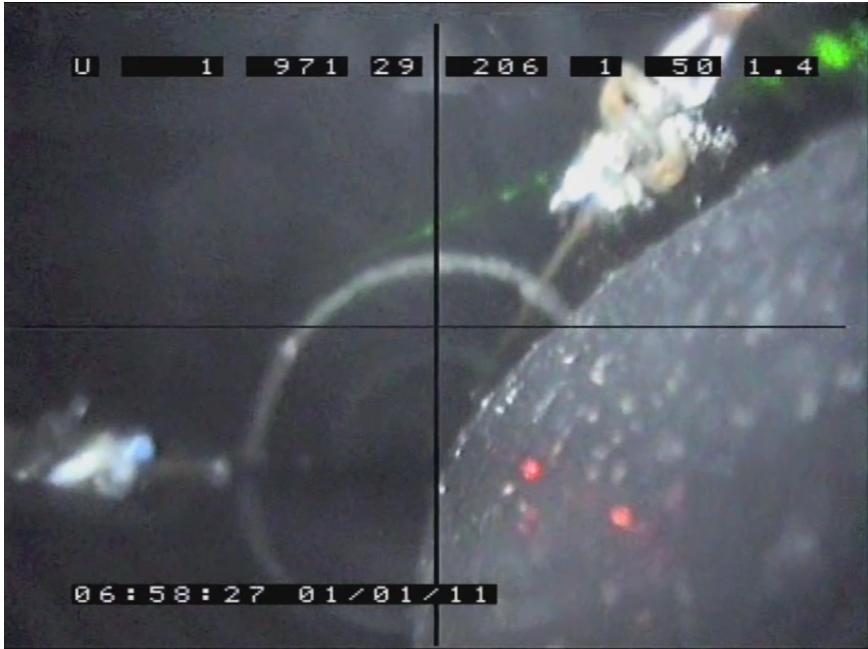
Figure 3.11 Photograph taken by a camera inside a DOM pressure vessel during the 2010-2011 deployment season, showing the clarity of the ice. The rings are spaced 1 meter apart. The green line is a calibration laser. The structure in the bottom right is ice refreezing after deployment.
