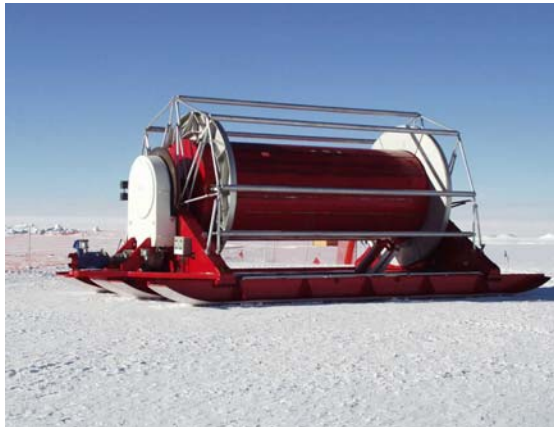
Figure 5. The hose-reel for the IceCube Hot Water Drill assembled at the South Pole, January 2004.
