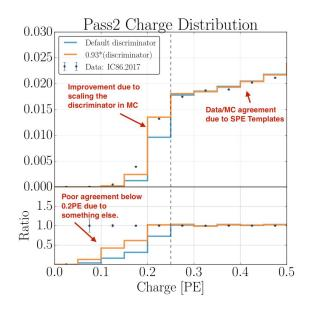
**Vuvuzela noise update**: The SPE Templates require an update to the noise. To reproduce the timing distribution of the noise, the noise is scaled by the area above the discriminator compared to the area above the discriminator of the TA0003 distribution. A comparison between the noise before and after the scaling is shown in red and yellow below, while the noise model used before the SPE templates is shown in green.
