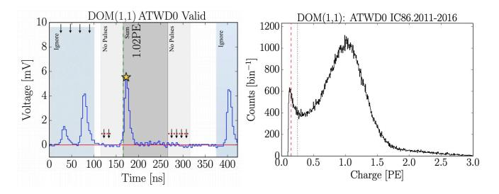
**Fig. 1:** Left: an illustration of the pulse selection. Set the 'pdf' option in SPE\_harvest.py to make these plots for every pulse. Right: the extracted charge distribution for DOM 1,1. You could make this plot after JSON files have been merged.
