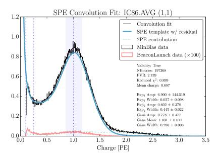
Fig. 6. An example output of the convolutional fitter for the ATWD, DOM 1,1 of all the years data summed together. The SPE Template is the red distribution. The semi-opaque region around the peak is where we prioritize the fitter. This is accomplished by minimizing the uncertainty in the data around the peak. The scipy fitting code has an option called sigma which allows you to specify the uncertainty.
