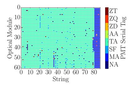
The majority of the standard QE DOMs have a TA identifier. The MA corresponds primarily to the HQE DOMs. The vertical lines in the plots below indicate DOMs which are instrumented with the old toroids.
