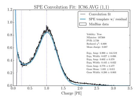
**Figure 5.** An example fit including the residual correction for DOM(1,1) using the WaveDeform dataset for seasons IC86.2011 to IC86.2016. The result from the convolutional fitter is shown as a solid black line. The extracted SPE template is shown blue.
