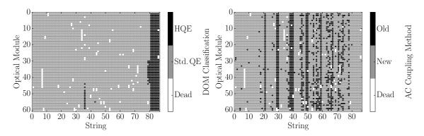
**Figure 1.** Left: A mapping of the HQE (black) and Standard QE DOMs (gray). Right: The version of AC coupling, old toroids (black) and new toroids (gray). DOMs that have been removed from service are shown in white.
