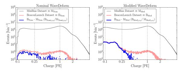
**Figure 3.** The cumulative charge distributions of all DOMs for the MinBias and BeaconLaunch datasets. The blue histogram shows the expected contribution from noise. This was found by subtracting the shape of the MinBias dataset from the BeaconLaunch dataset. Left: The charge distributions for the standard WaveDeform settings. Right: The charge distributions for the modified WaveDeform settings.
