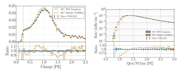
**Figure 9.** A comparison between the SPE templates (blue) and the TA0003 (orange) model for describing the SPE charge distribution in Monte Carlo. The simulation is compared to the 2012 IceCube season. Left: The total measured charge per DOM, per event at analysis level. Right: The distribution of the total measured charge of an event divided by the number of DOMs that participated in the event.
