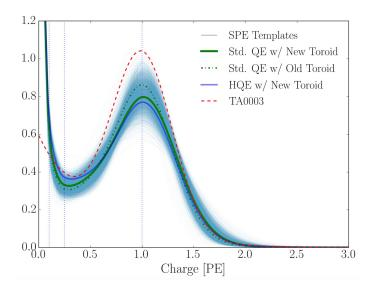
**Figure 7.** A comparison between the SPE templates (light blue band) and the TA0003 (dashed red line) distribution. The average SPE template for the Standard QE and HQE DOMs is shown as the thick blue and green lines, respectively. The SPE templates include the residual correction, and all curves are normalized.
