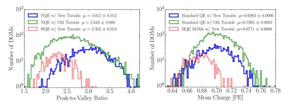
**Figure 6.** Comparison between the R7081-02MOD HQE DOMs and standard R7081-02 DOMs. Left: The peak-to-valley ratio for the two subsets of quantum efficiencies. Right: The mean charge of the individual DOM SPE templates.
