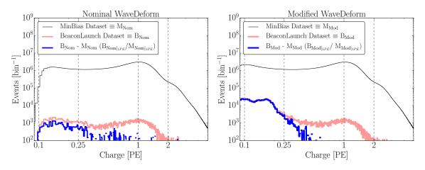
**Figure 3.** The cumulative charge distributions of all DOMs for the MinBias and BeaconLaunch datasets. The blue histogram shows the expected contribution from noise. This was found by subtracting the shape of the MinBias dataset from the BeaconLaunch dataset. Left: The charge distributions for the standard WaveDeform settings. Right: The charge distributions for the modified WaveDeform settings.
