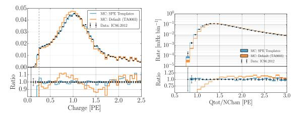
**Figure 9.** A comparison between the SPE templates (blue) and the TA0003 (orange) model for describing the SPE charge distribution in Monte Carlo. The simulation is compared to the 2012 IceCube season. Left: The total measured charge per DOM, per event at analysis level. Right: The distribution of the total measured charge of an event divided by the number of DOMs that participated in the event.
