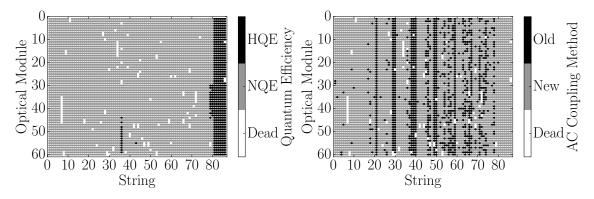
**Figure 1.** Left: A mapping of the HQE (black) and NQE DOMs (gray). Right: The version of AC coupling, old toroids (black) and new toroids (gray). DOMs that have been removed from service are shown in white.
