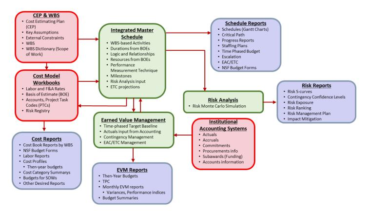
Figure 1: IceCube Upgrade project management flow diagram (based on the NSF Major Facilities Guide (3) Fig 4.2.2-1).
