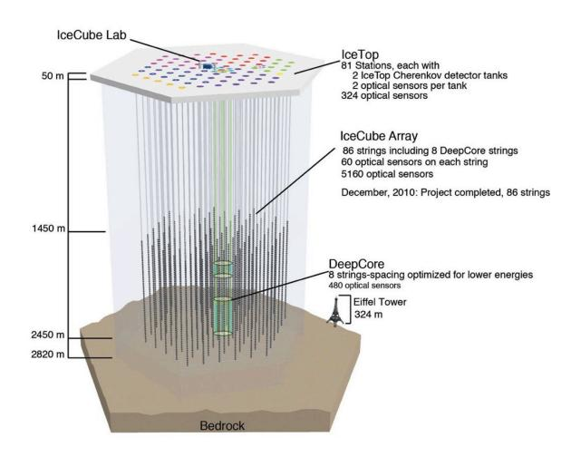
IceCube construction began in 2002 with design and procurement of the drill. The first string to be deployed was in Jan 2005. Over the next 6 season 85 more strings were deployed with the last string being "tied off" on December 17, 2010. Full 86 string data taking started May 2011.
