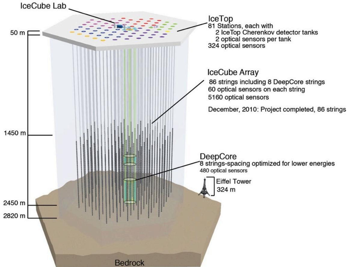
IceCube construction began in 2002 with design and procurement of the drill. The first string to be deployed was in Jan 2005. Over the next 6 season 85 more strings were deployed with the last string being “tied off” on December 17, 2010. Full 86 string data taking started May 2011.
