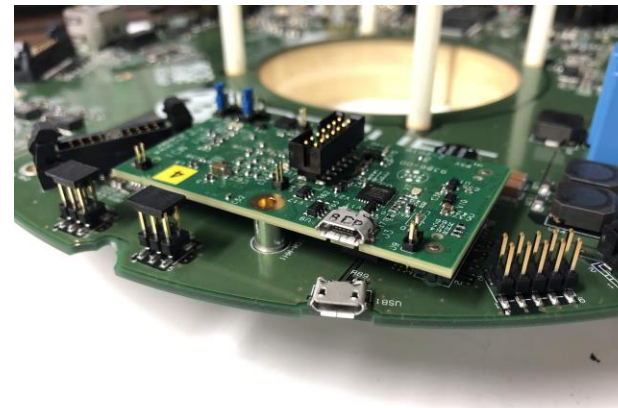
ICM mounted on D-Egg mainboard
