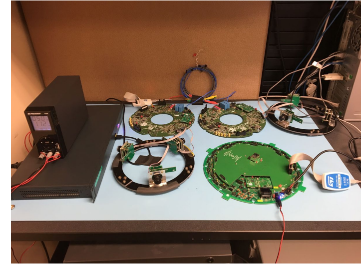
PCTS setup at UW mDOM and DEgg MBs
