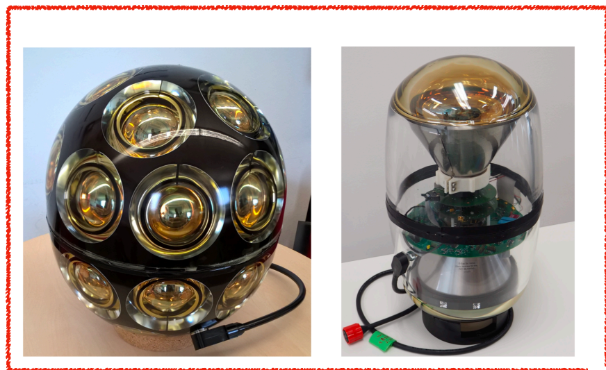
Directional information 24 x 3 inch PMT Diameter 36 cm
