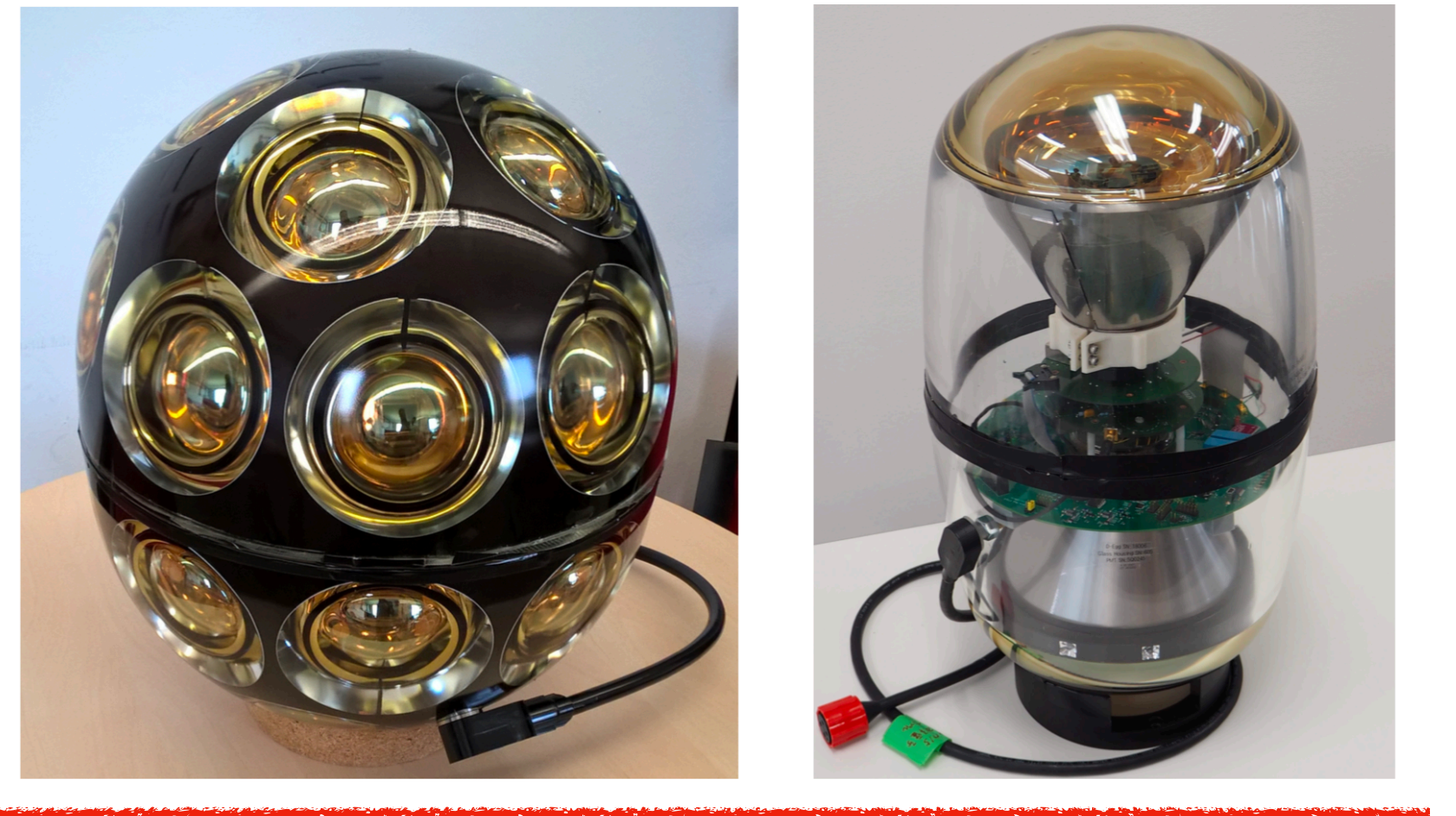
Directional information 24 x 3 inch PMT Diameter 36 cm
