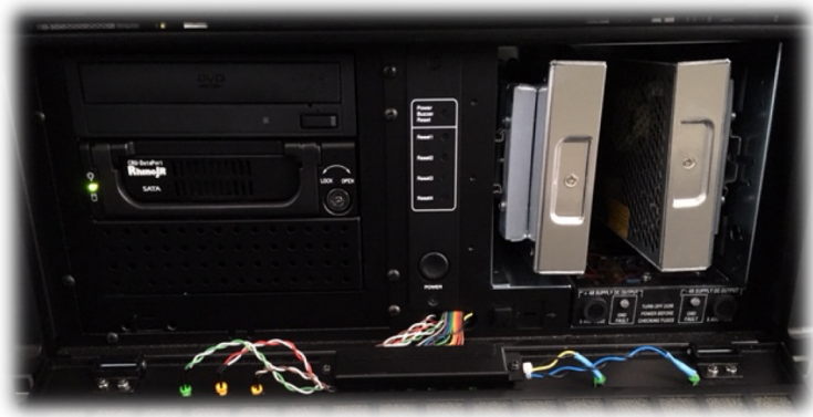
DOM power supplies tested at SPTS
