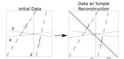
Figure 3: In this example, an event that is clearly composed of two muons (actual tracks shown as dashed lines) is treated as a single muon, and thus the reconstruction (sold line) is inaccurate.
