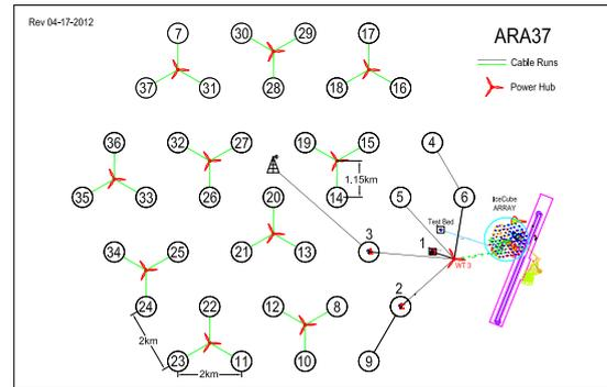
Figure 7: Example of the proposed ARA radio neutrino detector geometry: 37 stations would cover an area of about  $200 \text{ km}^2$  of ice. Hundreds of  $\text{km}^3$  of target volume are necessary to reach the desired sensitivities. See text for description of large radio detector configurations such as ARA and ARIANNA.
