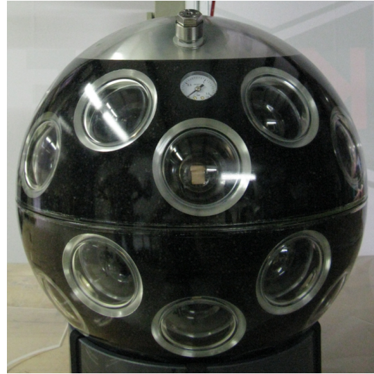
Figure 3: The optical sensor for KM3NeT contains 31 small PMTs (Photo [7])
