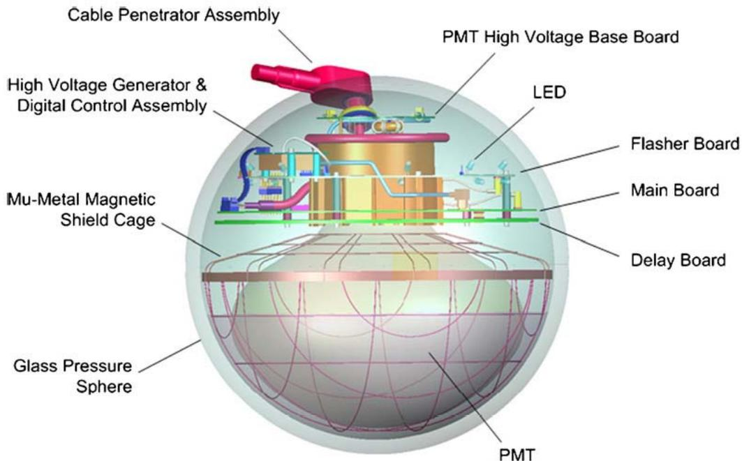
Fig. 3. A schematic view of an IceCube digital optical module.
