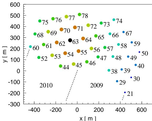
Figure 3: IceCube 40-string configuration as operated in 2008. String 63 (of DOMs that were used as flashers) is shown in black. IceCube parts installed in the following years (2009, 2010 as shown in the figure) lie in regions indicated approximately with dashed lines.
