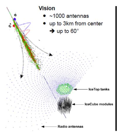
A radio array with an area of order 30 sq km as indicated in the figure would extend the maximum cosmic-ray energy accessible to ~5 EeV and would provide a considerable increase in the power of the surface array for vetoing EeV neutrinos. Before such an ambitious project can be contemplated, a smaller test demonstration project is needed.
