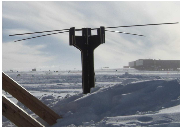
Fig. 5. Picture of the four arm dipole antennas MAPO1 and MAPO2. Every arm has a length of 0.7 m. The wooden stand is 1.2 m high. The final position of the antennas is the roof of the MAPO building.
