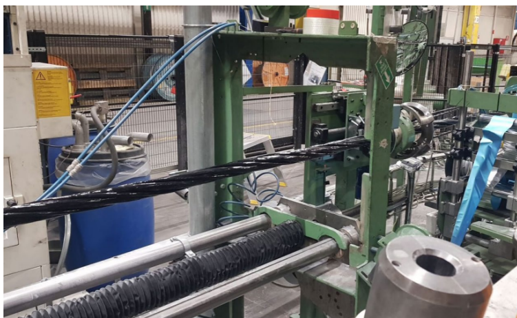
Figure 9: Test article of the main downhole cable being fabricated.
