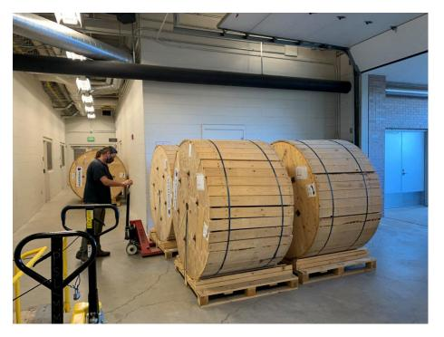
Main cable assembly temperature rating still to be verified – no vendor would guarantee storage temperature below -40°C but it is likely to be ok for a few days at temperatures below. (minimum temperature recorded in McMurdo is -56°C (-68.8°F) but it's very rare
