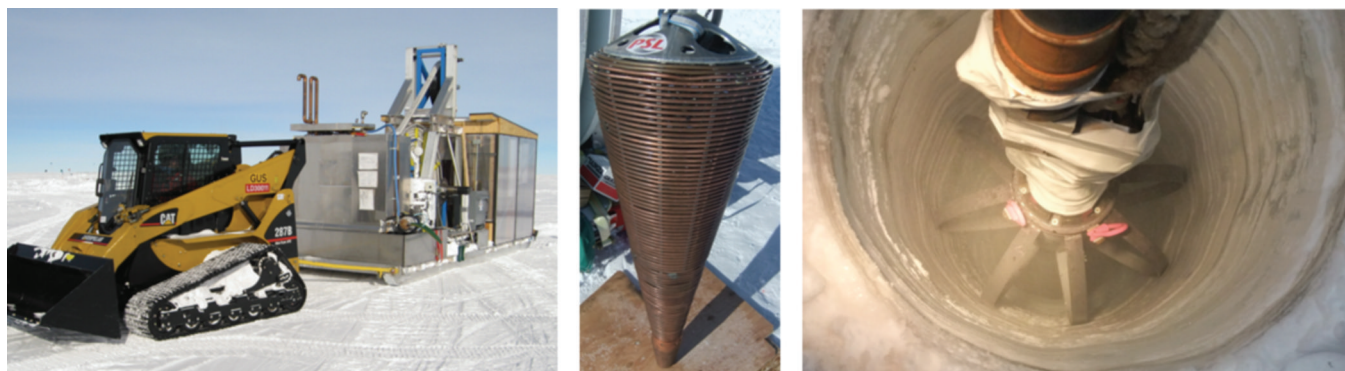
Fig. 5. (Left) independent firm drill sled; (middle) independent firm drill copper coiled cone; (right) IceCube drill head descending into a firm hole drilled by the independent firm drill.
