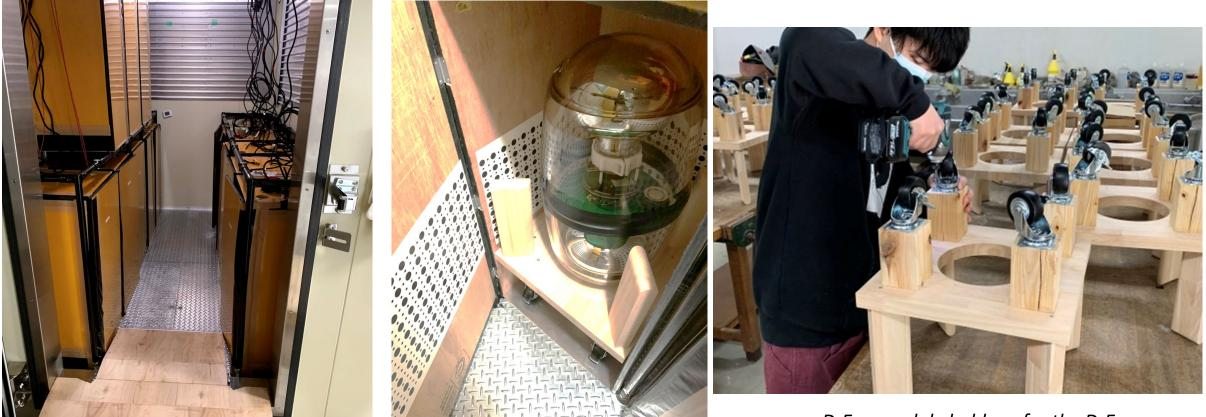
Freezer partially loaded with D-Eggs in their test structures
