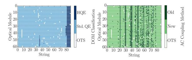
**Figure 1**. Left: A mapping of the HQE (dark blue) and Standard QE DOMs (light blue). Right: The version of AC coupling, old toroids (dark green) and new toroids (light green). DOMs that have been removed from service (OTS) are shown in white. These are primarily DOMs that resulted in failures during deployment and freeze-in, and failures during subsequent operation, as described in Ref. [9].
