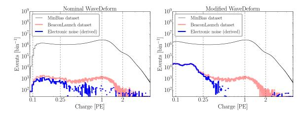
**Figure 3**. The cumulative charge distributions of all DOMs for the MinBias (M) and BeaconLaunch (B) datasets. The blue histogram shows the derived contribution from electronic noise. This was found by subtracting the normalized MinBias dataset from the BeaconLaunch dataset (B -  $M \times (B|_{IPE}/M|_{IPE})$ ). Left: The charge distributions for the standard WaveDeform settings. Right: The charge distributions for the modified WaveDeform settings.
