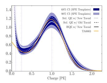
**Figure 8**. The inner (outer) dark blue region shows the 68% (90%) confidence interval defined by the measured spread in the extracted SPE charge templates of all DOMs in the detector. Superimposed are the average SPE charge templates for the variety of hardware configurations shown in white. The TA0003 distribution, for comparison, is shown in orange. All curves have been normalized such that the area above 0.25 PE is the same.
