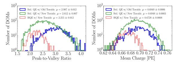
**Figure 6**. Comparison between the R7081-02MOD HQE DOMs and standard R7081-02 DOMs. Left: The peak-to-valley ratio for the two subsets of quantum efficiencies. Right: The average charge of the individual DOM SPE charge templates.
