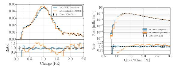
**Figure 9.** A comparison between the SPE charge templates (blue) and the TA0003 (orange) model for describing the SPE charge distribution in Monte Carlo. The simulation is compared to the 2012 IceCube season. Left: The total measured charge per DOM, per event at analysis level. Right: The distribution of the total measured charge of an event divided by the number of DOMs that participated in the event.
