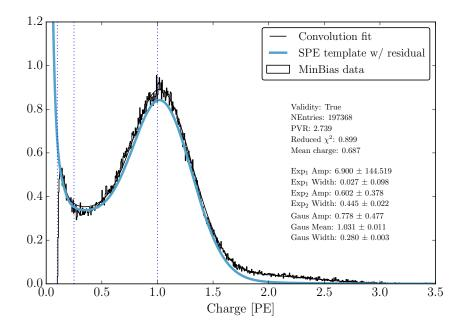
**Figure 5**. An example fit including the average residual from Fig. 4 for DOM(1,1) using the WaveDeform dataset for seasons IC86.2011 to IC86.2016. The result from the convolutional fitter is shown as a solid black line. The extracted SPE charge template is shown blue.
