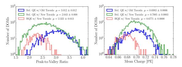
**Figure 6**. Comparison between the R7081-02MOD HQE DOMs and standard R7081-02 DOMs. Left: The peak-to-valley ratio for the two subsets of quantum efficiencies. Right: The mean charge of the individual DOM SPE charge templates.
