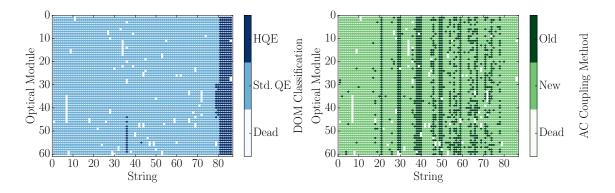
**Figure 1**. Left: A mapping of the HQE (dark blue) and Standard QE DOMs (light blue). Right: The version of AC coupling, old toroids (dark green) and new toroids (light green). DOMs that have been removed from service are shown in white.
