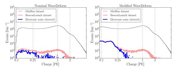
**Figure 3**. The cumulative charge distributions of all DOMs for the MinBias (M) and BeaconLaunch (B) datasets. The blue histogram shows the derived contribution from electronic noise. This was found by subtracting the normalized MinBias dataset from the BeaconLaunch dataset (B -  $M \times (B|_{1PE}/M|_{1PE})$ ). Left: The charge distributions for the standard WaveDeform settings. Right: The charge distributions for the modified WaveDeform settings.
