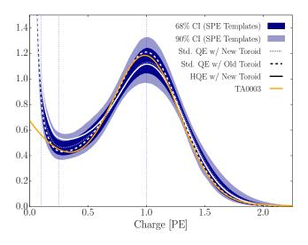
**Figure 7.** The inner (outer) dark blue region shows the 68% (90%) confidence interval defined by the measured spread in the extracted SPE charge templates of all DOMs in the detector. Superimposed, is the average SPE charge template for the variety of hardware configurations shown in white. The TA0003 distribution is shown in orange. All curves have been normalized such that the area above 0.25 PE is the same.
