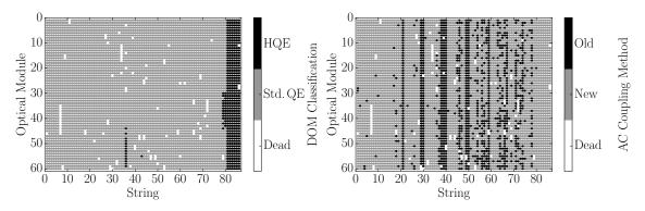
**Figure 1.** Left: A mapping of the HQE (black) and Standard QE DOMs (gray). Right: The version of AC coupling, old toroids (black) and new toroids (gray). DOMs that have been removed from service are shown in white.
