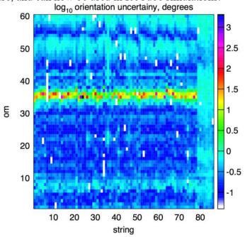
Figure 1: The error on the reconstructed position of LED 7 in degrees for all IceCube DOMs. The uncertainty is better than 1° for most DOMs, except in the dust layer where the optical properties are poor.
