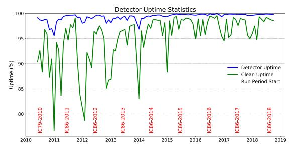
Figure 1: Total IceCube Detector Uptime and Clean Uptime
