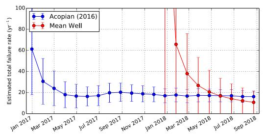
Figure 3: Estimated full-detector failure rate of the two types of DOM power supplies in use.
