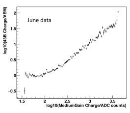
Figure 6: Air shower charge in scintillator panel (x-axis) vs. IceTop Tank 43B (y-axis)
