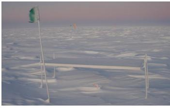
Figure 5: Elevated scintillator panel in operation after the 2018 winter.
