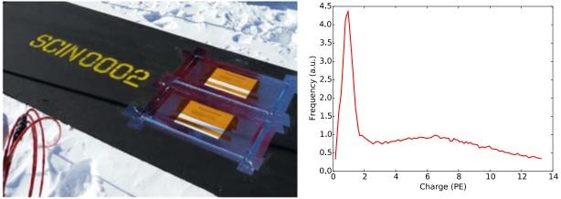
Figure 5: Left: Scintillator deployed over IceTop station 62. Right: Charge spectrum of scintillator, showing single photoelectron peak at 1PE and broad cosmic-ray muon peak at ~6PE.
