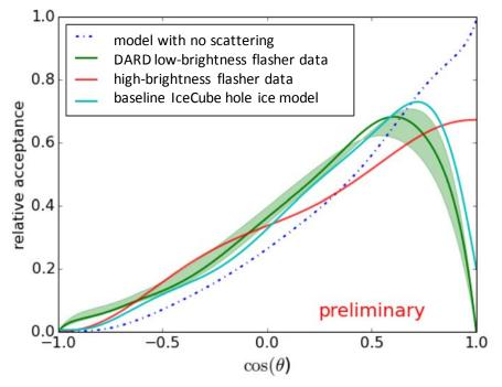
Figure 2: Hole ice effect on DOM relative acceptance as a function of incident photon zenith angle from various studies including: low-brightness flashers in ice (DARD); a multi-parameter fit to bright flasher data; and the simulation-based default hole ice model.
