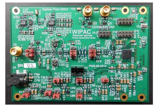
Analog/digital front end boards fabbed 2015Q1 – good performance – 250 MSPS 14-bit, < 300 mW. Noise at 2 LSB. Plug-in via HSMC to standard FPGA development board. *P. Sandstrom - WIPAC*
