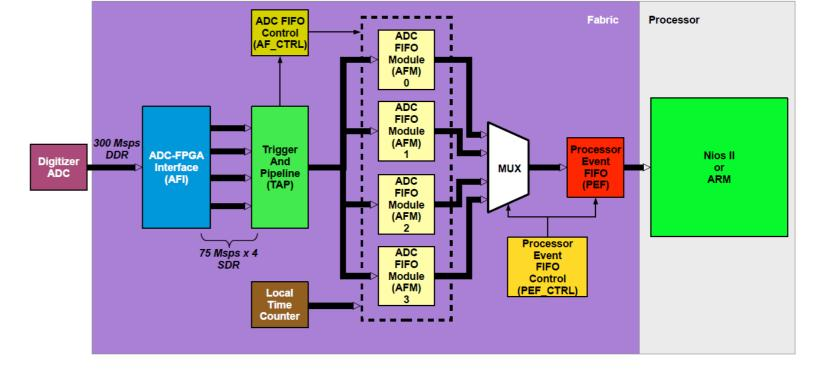
Early prototype firmware with advanced features: full throughput at 250 MSPS (quad pipeline) and control via soft core Nios on Cyclone V FPGA.
