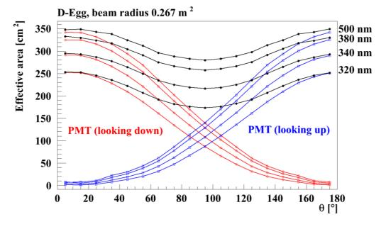
D-Egg uses 2x 8" PMTs. Naively, one would expect only about 30% enhancement in the photon effective area, however, better collection efficiency relative to 10" PMT and massive improvements in UV transparency of glass.
