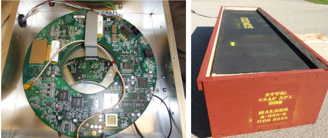
**Figure 6: Left: Spare DOM mainboard integrated into a prototype scintillator. Right: Modules crated for shipment from UW Physical Sciences Laboratory.**
