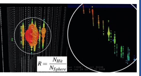
Each event was split into two halves  $(t_1, t_2)$  based on the charge-weighted mean time, and the cascade reconstruction was run on each half separately. Then, the difference TimeSplitPosition between reconstructed vertex positions for both halves was calculated. For the events consistent with a signal cascade hit pattern this number has a smaller value than for track-like events.
