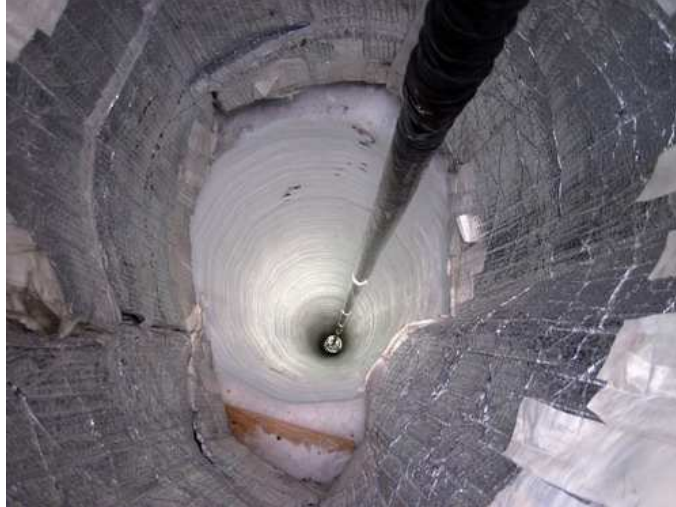
Figure III.2: Sensor descends down a hole in the ice as part of the final season of IceCube deployment
