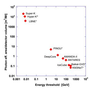
Figure 4: The effective photodetection area per unit mass is plotted versus the approximate energy threshold of various water/ice Cherenkov detectors. Detectors that are in a planning or a conceptual phase are indicated with an (\*). The effective PMT coverage scales roughly to the inverse of the threshold for a wide range of detectors. There are no existing detectors with intermediate thresholds in the range 0.1 to 10 GeV.
