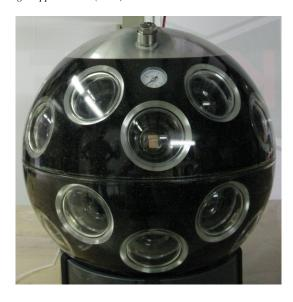
Figure 3: The optical sensor for KM3NeT contains 31 small PMTs (Photo courtesy KM3NeT[8])
