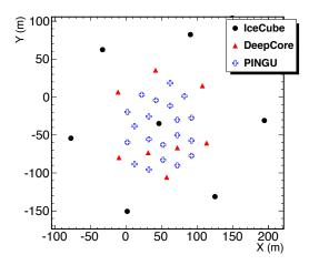
Figure 5: Possible geometry of a low energy infill detector PINGU with 20 additional strings instrumenting 5 Mtons of ice in the center of IceCube. An instrumented detector of that scale has the potential to determine the mass hierarchy of neutrinos using upward going atmospheric neutrinos.
